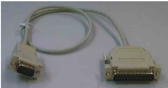
Fig.1 ISP CABLE :12NC IS "3138 106 10148".
